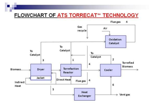
The above Flowchart provides an example configuration of a torrefaction system using ATS TorreCat<sup>™</sup> Technology.
